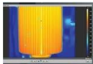
Infrared picture of super conductor after lighting for about 30 minutes
